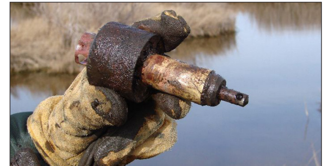
U.S. Army Corps of Engineers Remedial Investigation team removes a World War I MK-I fuze from Plum Tree Island Range. (USACE Photo)
